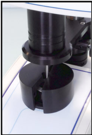
Thermal Enclosure, for use on all systems. Designed to insulate the sample from the environment.
